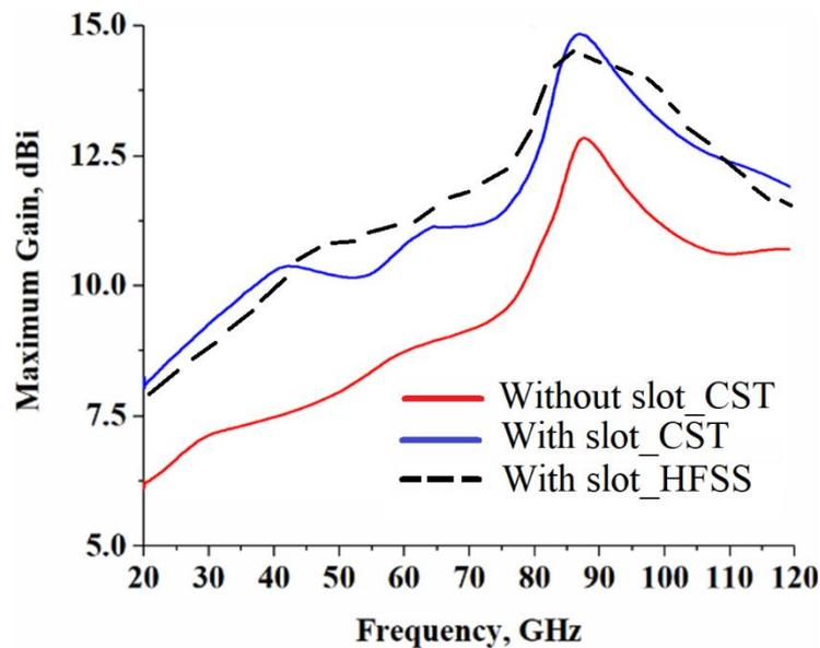
Figure 4. Gain response for both cases “with no” slot and “with” slot using two different commercially available 3D full wave electromagnetics simulation tools (CST Microwave Studio® and HFSS™).
