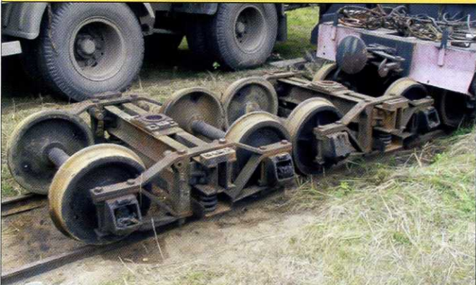
Diamond frame bogies with coil springs at Talitsy (Pereslavl Railway Museum).
