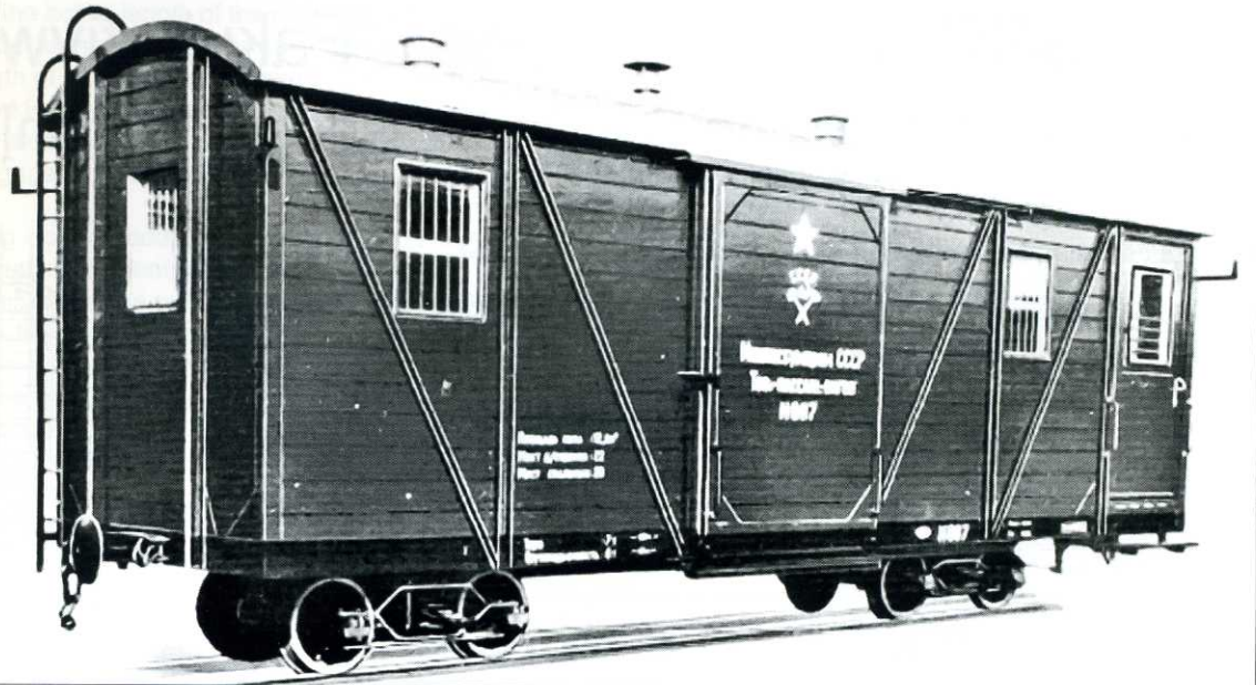
Works picture of the exterior of a USSR Fakultativwagen. Ammendorf Works
