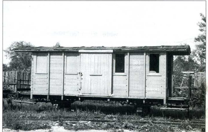
Former German 'Reparations' 0.750m Fakultativwagen in use on the Shatura peat railway network in the 1980s.
