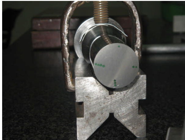
Figure 3.17: The position of (green marked) for surface roughness checking
