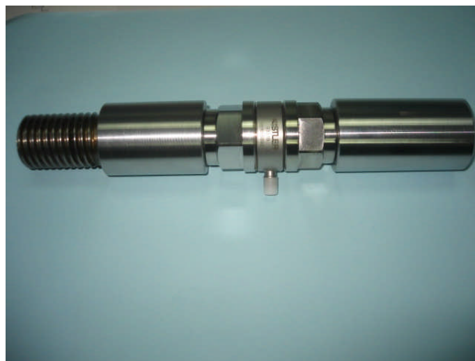
Figure 3.26: Ejector rod and Kistler's link assembly
