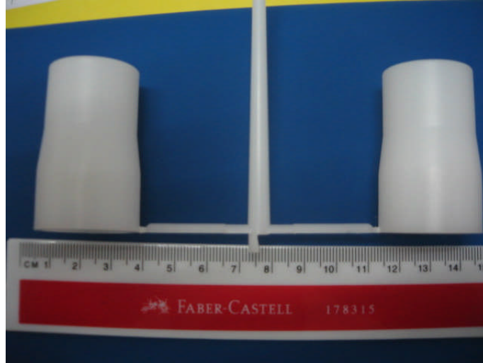
Figure 5.2: Part sample of HIPS
