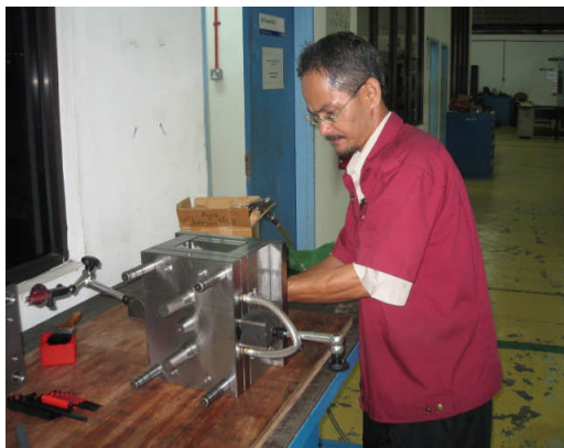
(n) Fitting Test mould
