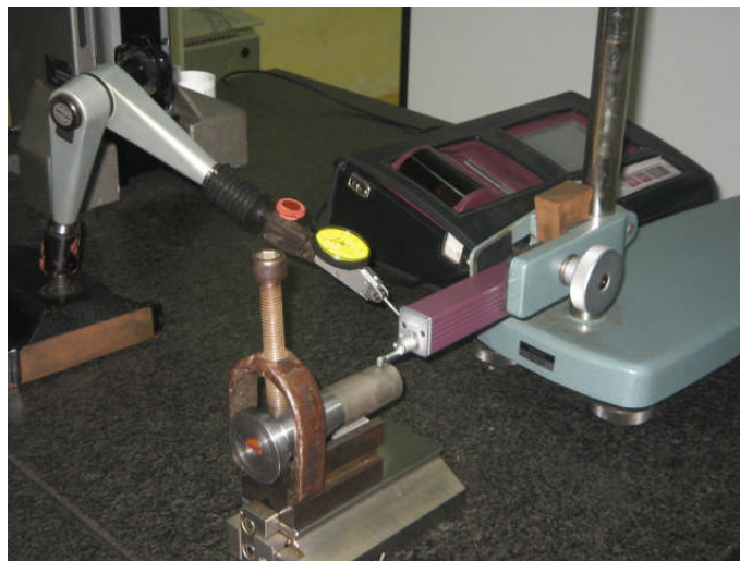
Figure 3.18: The layout equipment set-up for checking the surface roughness for core inserts
