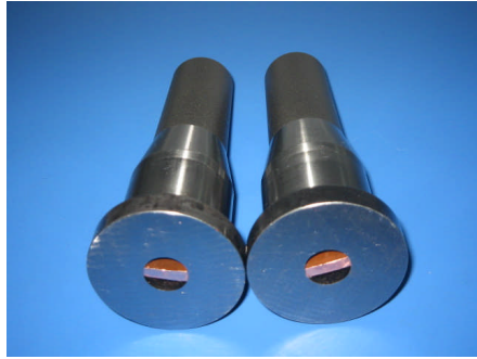
(a) Core insert with copper plate inside
