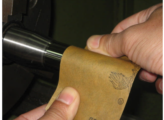
(b) Applied different grade of sand paper
