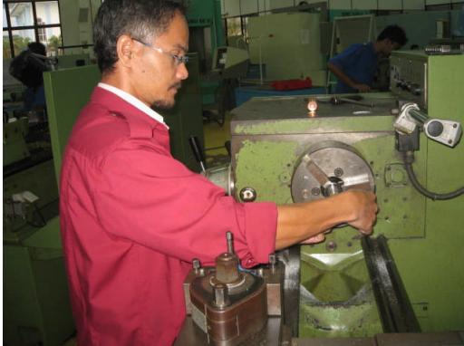
(a) Setting up the insert on the machine
