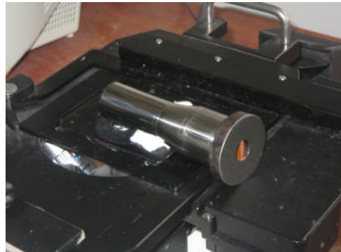
(c) Positioning polished core insert
