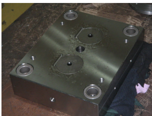
(h) Fitting 2 cavity inserts and dowel pins
