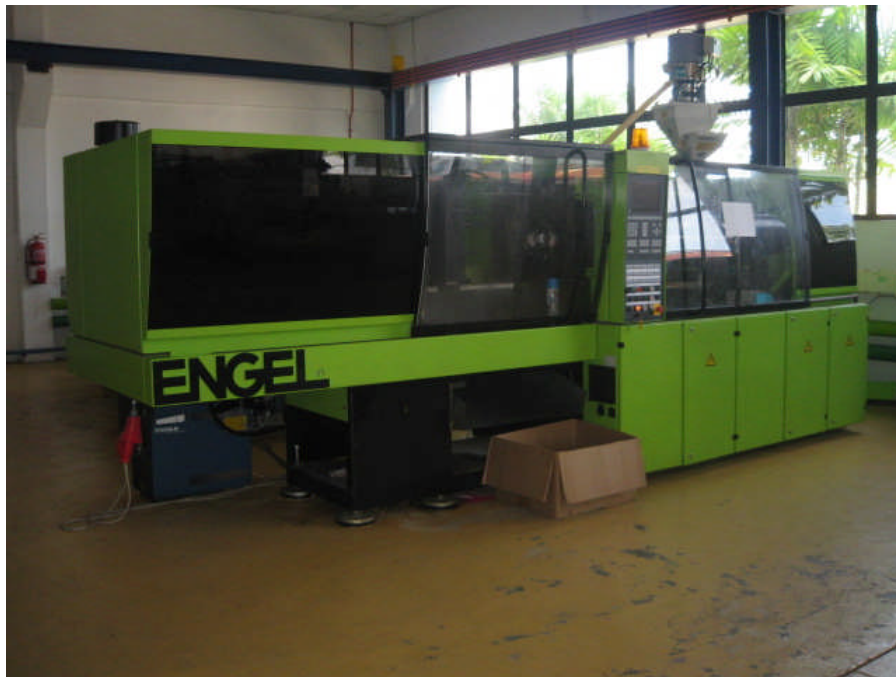
Figure 3.23: An Engel injection moulding machine (HLV-125)
