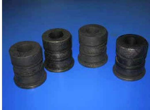
(b) Cavity insert after heat treatment
