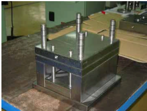
(d) Some of mold base parts waiting for machining
