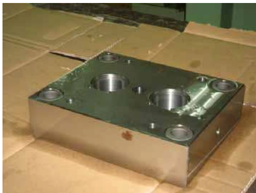
(f) After machining process for cavity plate
