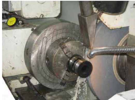
(b) Cylindrical grinding (CG) process for cavity insert
