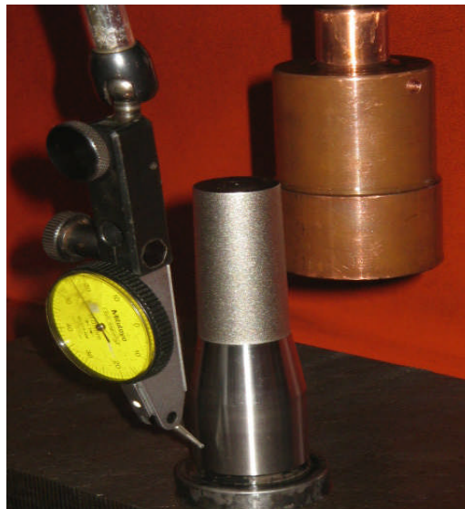
(c) Surface roughness after EDM process
