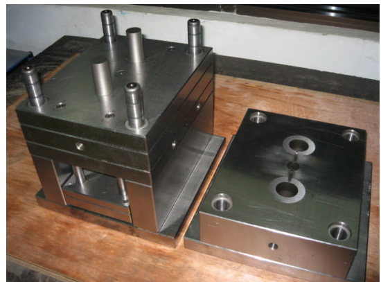
(o) Test mould in open position
