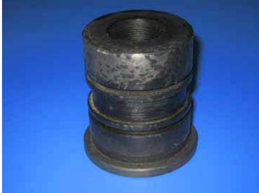
(a) Cavity insert after heat treatment
