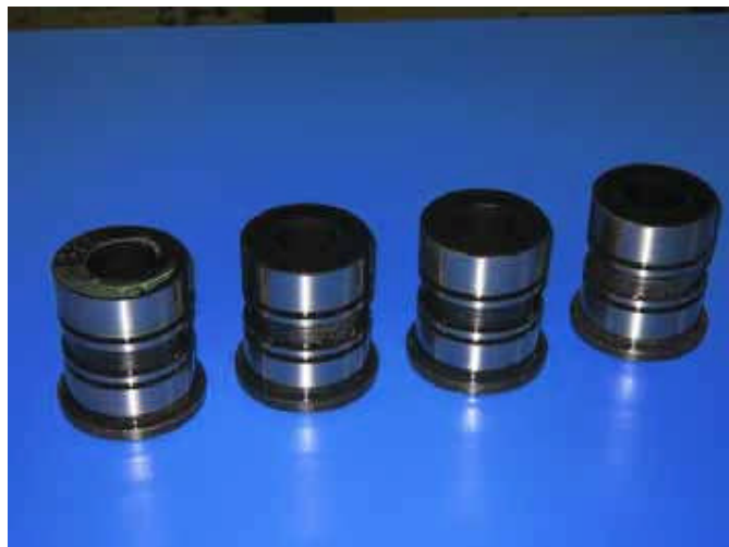
(c) After OD (out side diameter) machining
