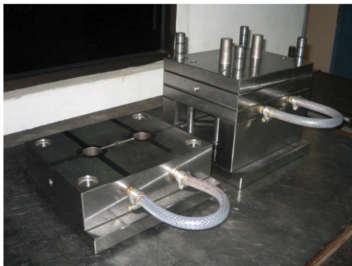
Figure 3.22: Test mould ready for trial out
