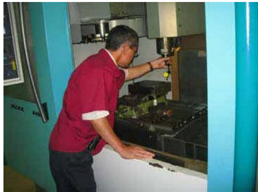
(e) Setting cavity plate prior machining process
