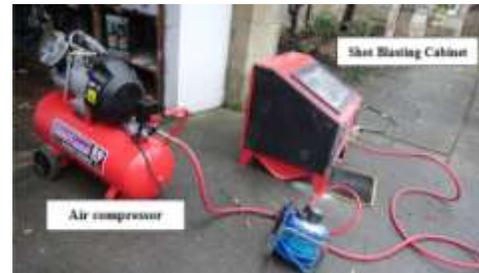
Figure 2. The abrasive cleaning system.
