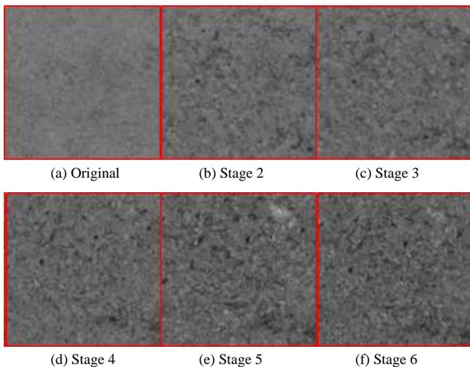
Figure 10. Greyscale images of yellow clay brick cleaned with medium glass at cleaning stages 1 to 6.
