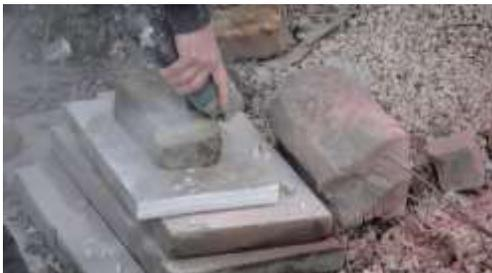
Figure 1. Cutting samples from original stones and bricks.
