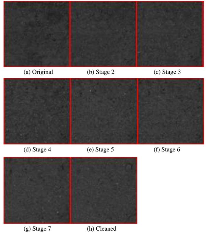
Figure 11. Greyscale images of red clay brick cleaned with medium glass at cleaning stages 1 to 8.
