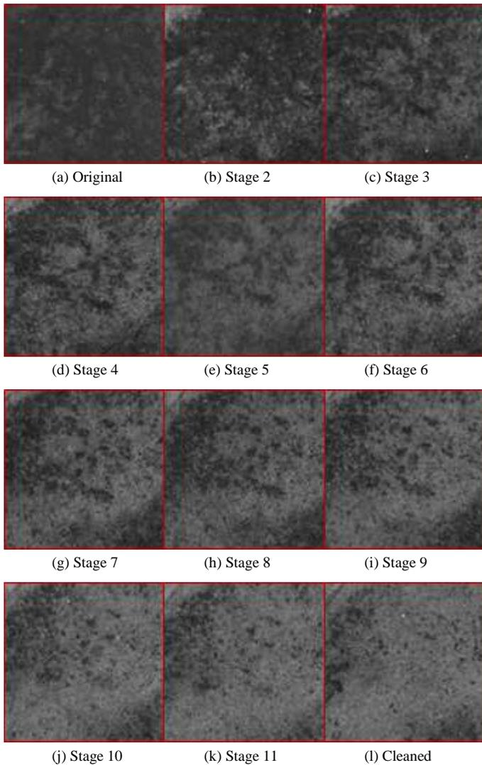
Figure 9. Greyscale images of red sandstone cleaned with fine glass at cleaning stages 1 to 12.
