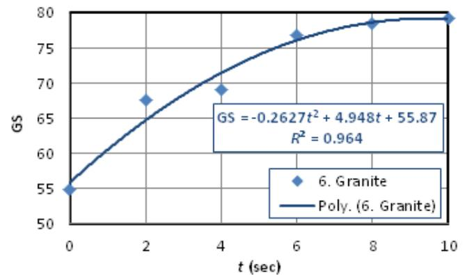
Figure 12. Greyscale versus cleaning time for granite cleaned with fine glass.
