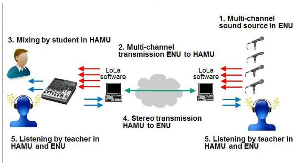
Figure 3.2: The scenario of the remote sound mixing experiment between AMU (Prague) and ENU (Edinburgh)
