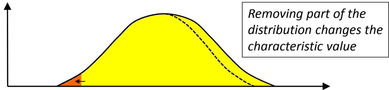
If the cross-section of the timber is reduced, this changes the influence of knots, sloping grain and other characteristics. EN14081 has a limit on reprocessing. The reason for this limit still holds at the fabricator and on the construction site.
