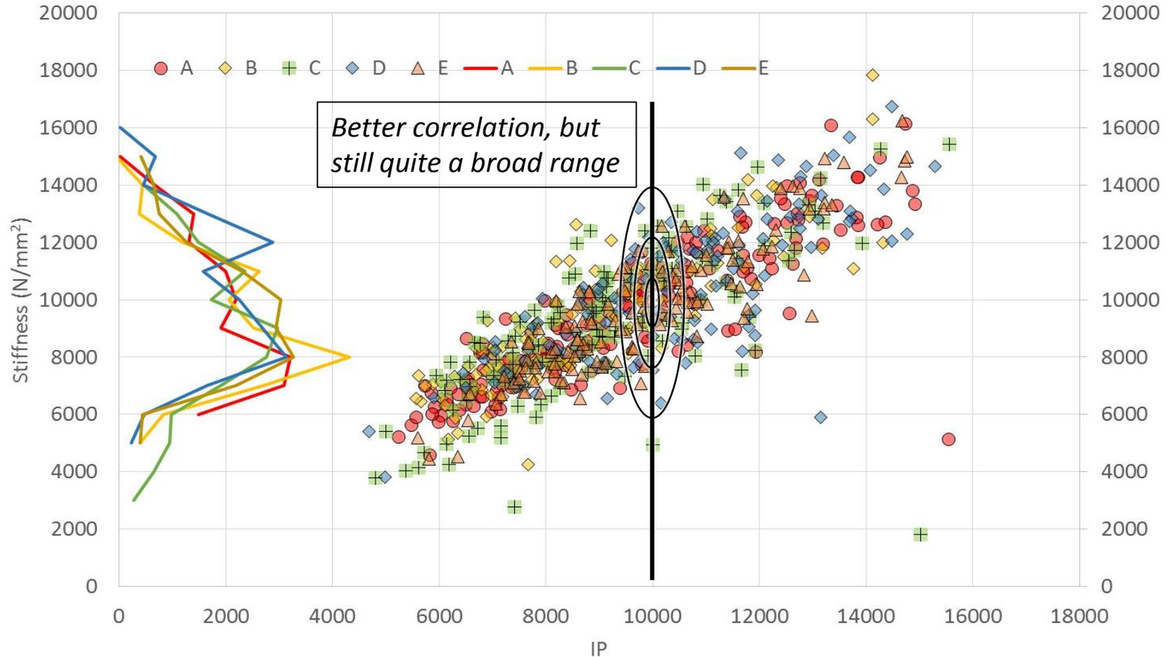
(Dynamic modulus of elasticity from longitudinal resonance)
