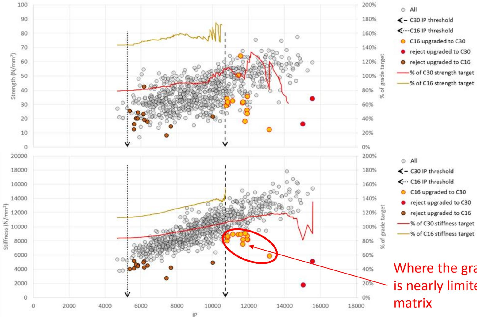
Where the grading process is nearly limited by the cost matrix
