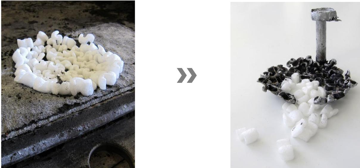
Fig: 1. Polystyrene packaging pellets as a waste mould (left) for a sand-cast aluminium bowl (right). Author 2015
