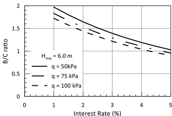
Figure 8: Benefit/Cost (B/C) ratio against Interest Rate (%) for ground improvement depth  $H_{imp} = 6$  m and three different applied foundation pressures  $q$  (kPa).
