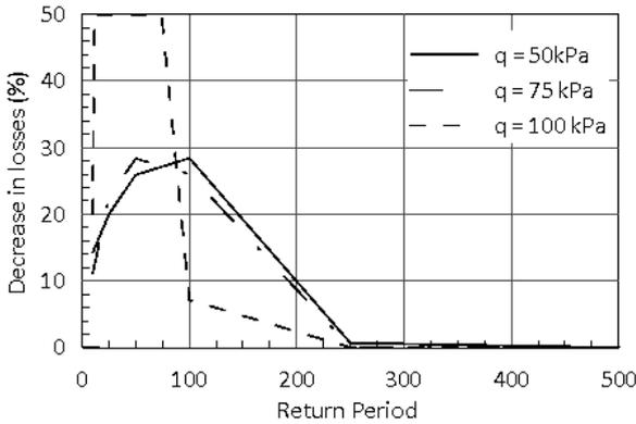
Figure 5: Percent decrease in anticipated losses from increasing the ground improvement depth  $H_{imp}$  from 4 to 6 m.
