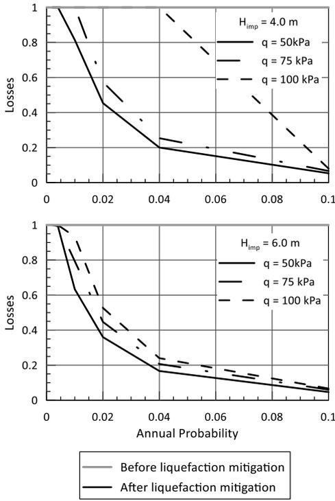
Figure 4: Losses before and after ground improvement for two ground improvement depths  $H_{imp} = 4$  &  $6$  m and three applied foundation pressures  $q$  (kPa).
