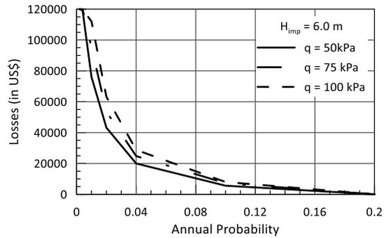
Figure 6: Losses in monetary values (US\$) for ground improvement depth  $H_{imp} = 6 \text{ m}$  and three applied foundation pressures  $q$  (kPa).
