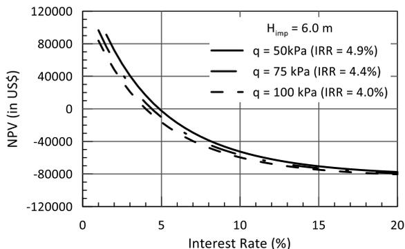
Figure 7: Net Present Value (NPV) against Interest Rate (%) for ground improvement depth  $H_{imp} = 6$  m, and three different applied foundation pressures  $q$  (kPa).
