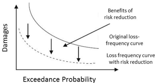
Figure 1: Benefits of DRR in shifting the loss-exceedance curve.
