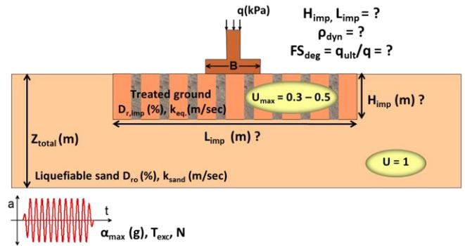
Figure 2: Typical configuration of the proposed foundation scheme of shallow foundations on top of liquefiable soils with prior ground improvement with the use of gravel drains.
