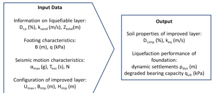
Figure 3: Flow chart with the required information for the application of the proposed methodology.
