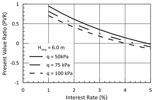
Figure 9: Present Value Ratio (PVR) against Interest Rate (%) for ground improvement depth  $H_{imp} = 6$  m and three different applied foundation pressures  $q$  (kPa).
