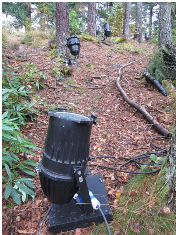
Fig.1 The standard approach for lighting temporary night time events in woodlands is to use theatrical equipment such as these 1kW Par cans uplighting pine trees. Why is so much light required?
