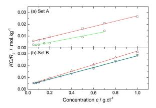
**Fig. 8** *Kc*/ $R_{\theta}$  obtained using static light scattering has been plotted against concentration for **a** HEC (*open square*) and hmHEC (*open circle*) in set A and **b** hmHEC-Blank (*open triangle*), hmHEC-1 (*open inverted triangle*) and hmHEC-2 (*open star*) in set B. The data points for each polymer have been fitted with straight lines in order to calculate second virial coefficient ( $A_2$ ) values according to Debye equation. (Color figure online)
