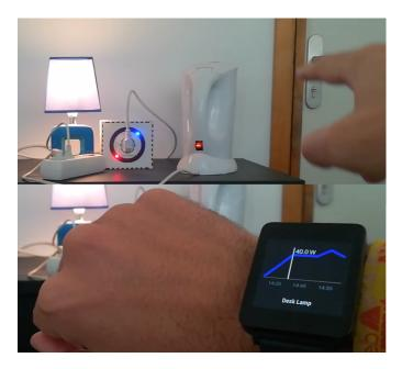
Fig. 3. Wattom's NILM capabilities enables the user to interact with various concurrent appliances connected to a single plug. In this example the lamp and kettle are represented by a blue and red targets, respectively (top). Upon selection, Wattom displays a plot with the consumption of the appropriate appliance in the user's smart watch (bottom).
