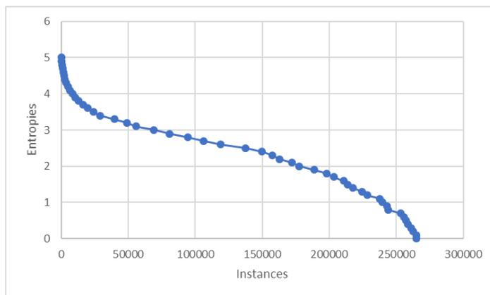
Figure 5: Typical Memory Segment Entropy Distribution
