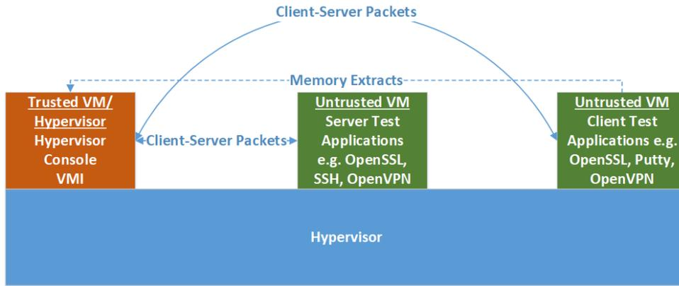
Figure 3: *MemDecrypt* Virtualization Architecture
