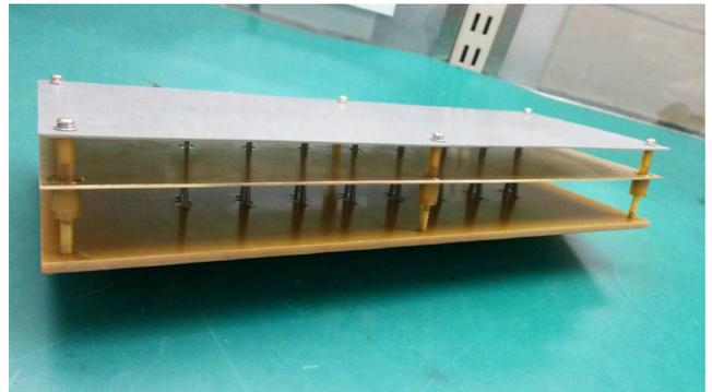
**FIGURE 10.** The prototype of the 1 × 8 linear phased array with the proposed balun.
