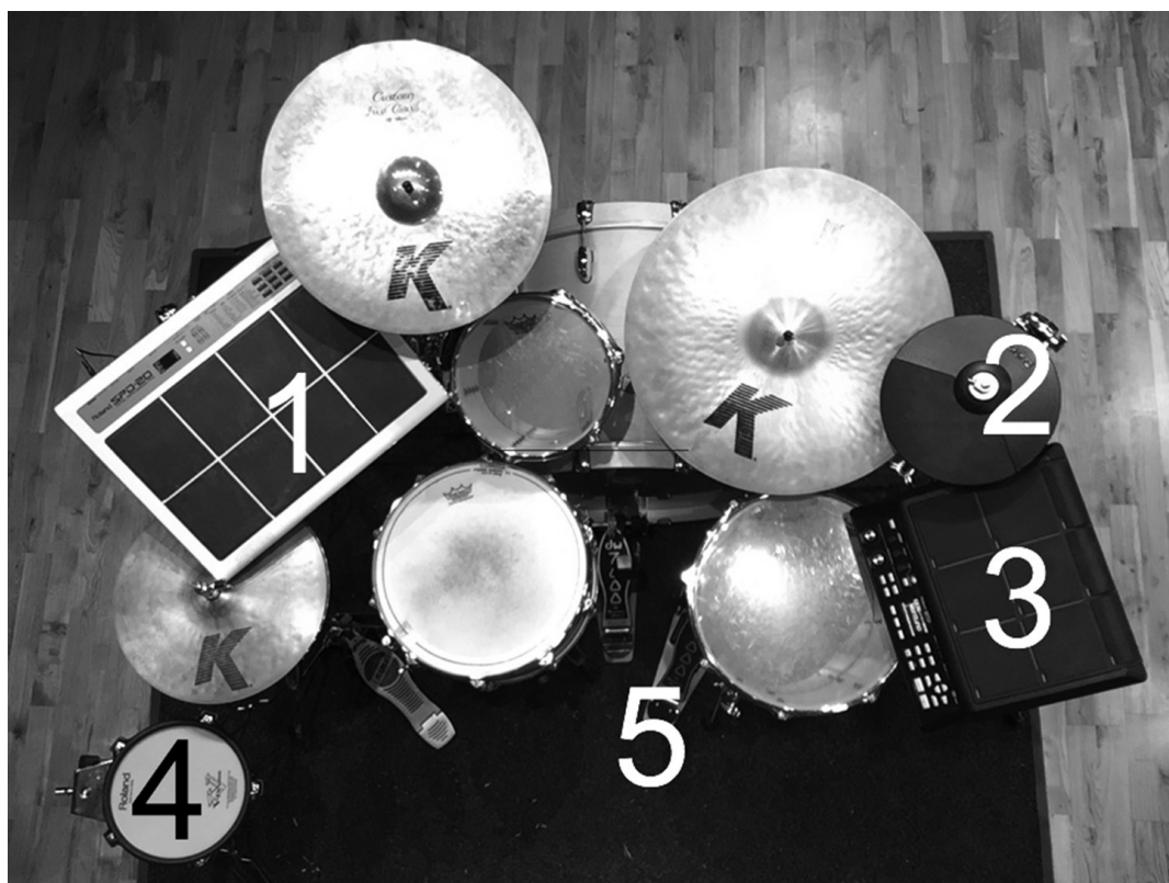
Figure 13.1 A hybrid drum kit setup containing: (1) Roland SPD-20 percussive controller, (2) Roland CY-5 cymbal trigger pad, (3) Roland SPD-SX sample pad, (4) Roland PD-85 mesh head trigger pad, and (5) Roland KD-7 kick drum trigger.
