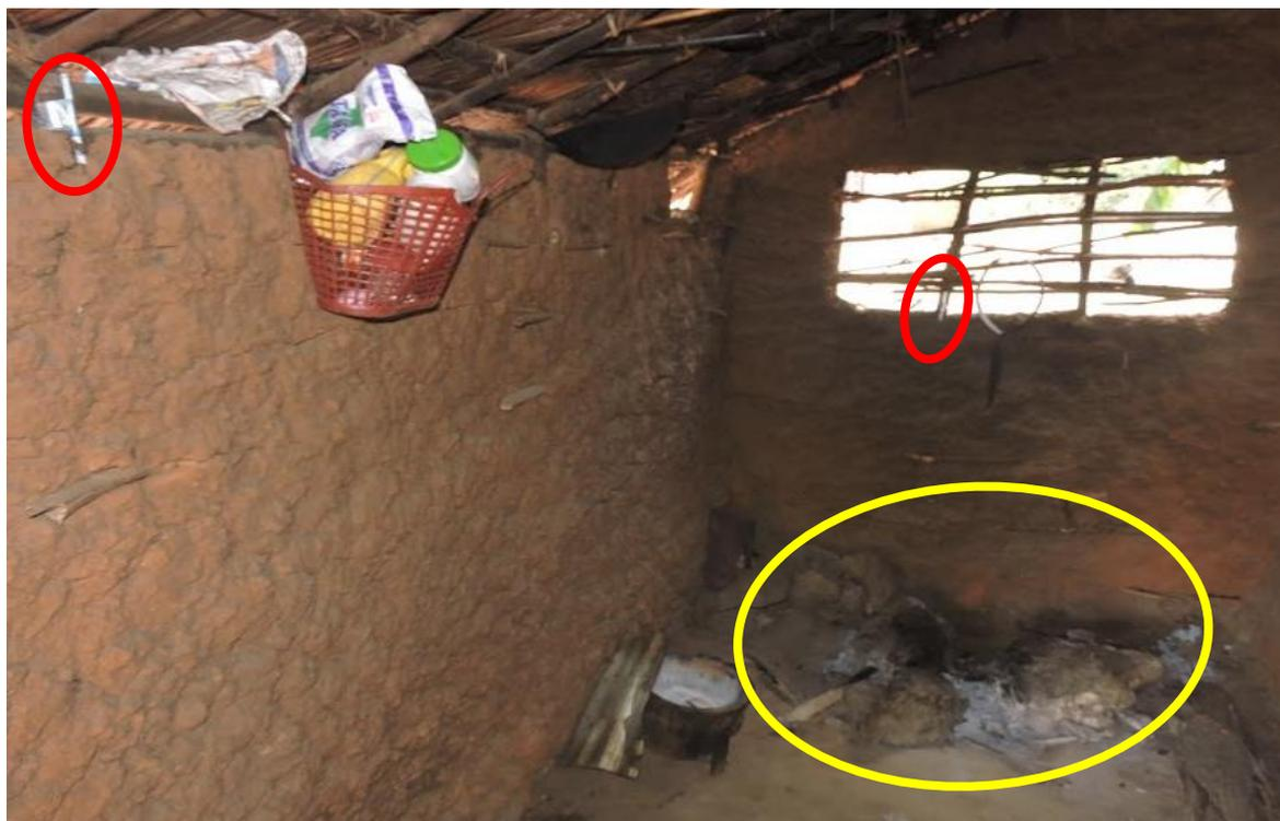
**Figure 2:** Sampling setup for CO passive diffusion tubes. Red circles indicate location of Dosi tubes, the yellow circle shows the three-stone fire.
