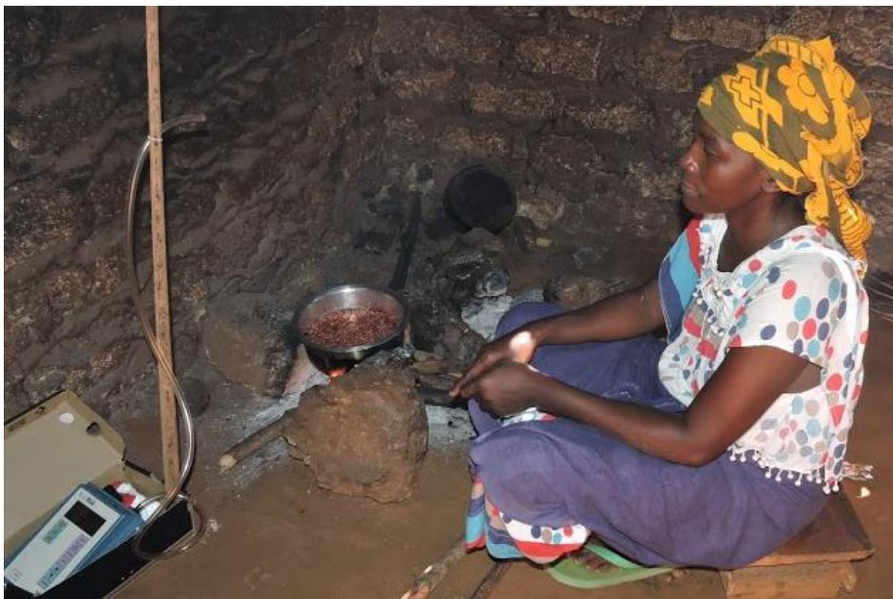
**Figure 4:** Sampling setup to measure PM<sub>2.5</sub> during the cooking process in households.
