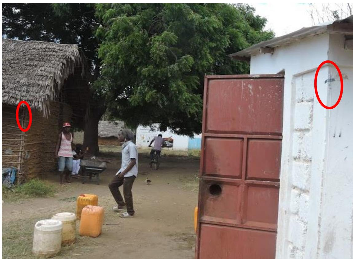
**Figure 3:** Sampling arrangement for the ambient CO measurements with the passive diffusion tubes. Red circles indicate the locations of the tubes.
