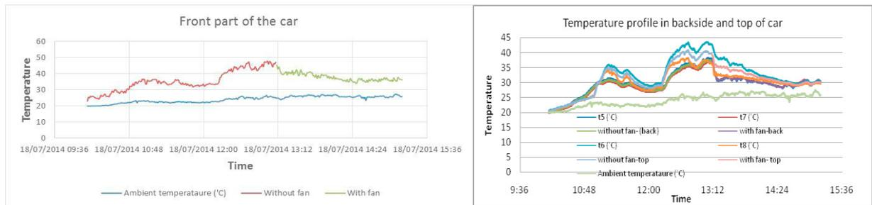
Fig 12: Temperature profile in front, back and topside of the car (without and with fan) [1]
