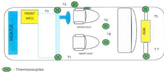
Fig 2. The thermocouples positions in the car
