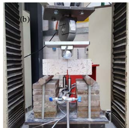
Fig. 3. (a) Three-point bending test configuration; (b) actual test set-up (200mm span).
