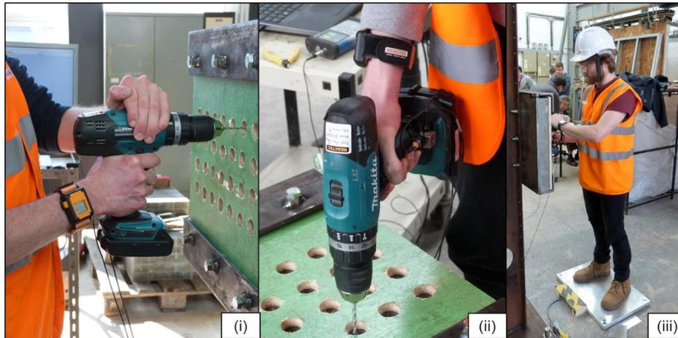
**Figure 2** Test postures (i) horizontal (ii) vertical downwards and (iii) force plate location.
