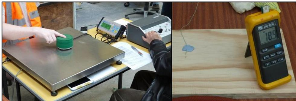
**Figure 2** VPT assessment using vibratory sensation meter (Rion Company Ltd. Model AU-02A) and skin temperature thermocouple sensor (RS 206-3738).
