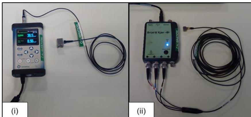
**Figure 3** Tool emission instrumentation (i) Svantek SV106 & SV 150 accelerometer (ii) Brüel & Kjær Photon+ 4520-001 accelerometer.
