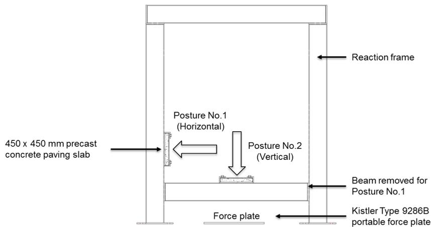
**Figure 1** Reaction frame configuration showing postures and force plate location.
