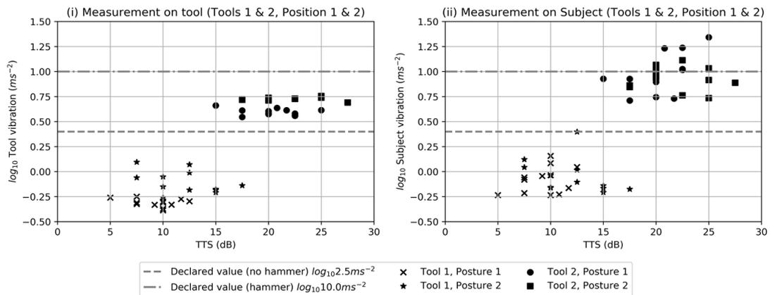
**Figure 5** TTS vs (i) tool and (ii) subject vibration measurements for all tests. Manufacturers declared emission values of 2.5  $\text{ms}^{-2}$  and 10.0  $\text{ms}^{-2}$  provided for reference purposes
