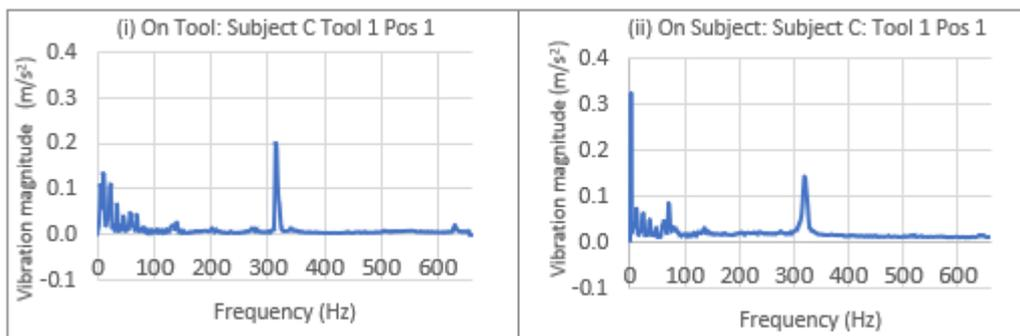
**Figure 4** Tool setting No.1 (drill), posture 1 – (i) frequency response on tool and (ii) frequency response on subject.
