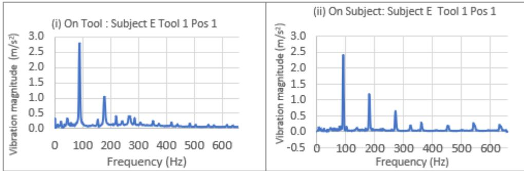
**Figure 5** Tool setting No.2 (impact drill) – (i) frequency response on tool and (ii) frequency response on subject.
