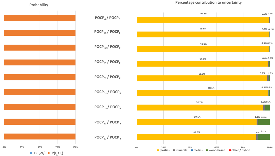
FIGURE O.12 Estimated uncertainties associated with the comparisons of timber buildings with reference building F, for POCP. Indication of probability (left) and relative contribution to uncertainty (right).
