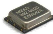
The **Model 832M1** is a low cost, board mountable triaxial accelerometer. Featuring stable piezo-ceramic crystals, the accelerometer incorporates full power and signal conditioning with a maximum current consumption of 22 micro-amps. The model 832M1 is available in  $\pm 25\text{g}$  to  $\pm 500\text{g}$  ranges and provides a flat frequency response up to greater than 6kHz. The standard model 832 offers the same envelope with a lower maximum current consumption of 4 micro-amps.
