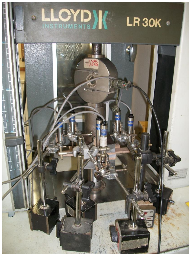
Fig (8) Compression test apparatus with measurement transducers.
