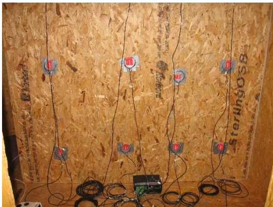
Fig. (16) Sensor equipment during calibration.
