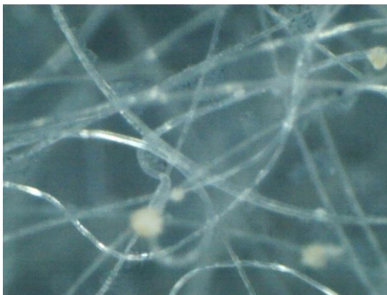
Figure 3. Magnified image of the aerogel surface.
