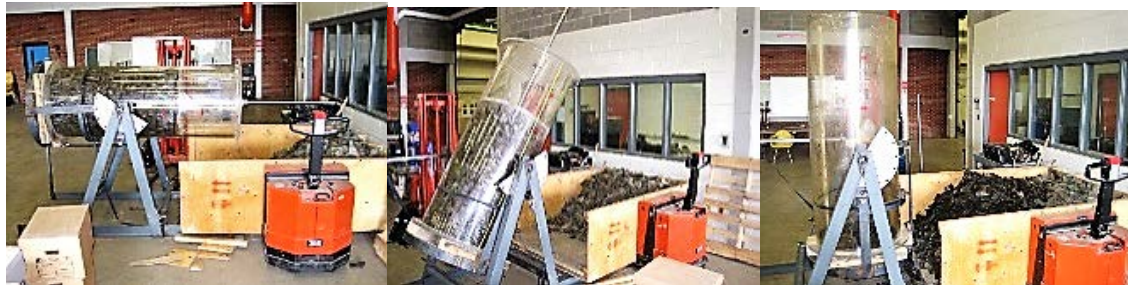
FIG.4 Gantry system for unloading and loading the consolidometer outside the load frame
