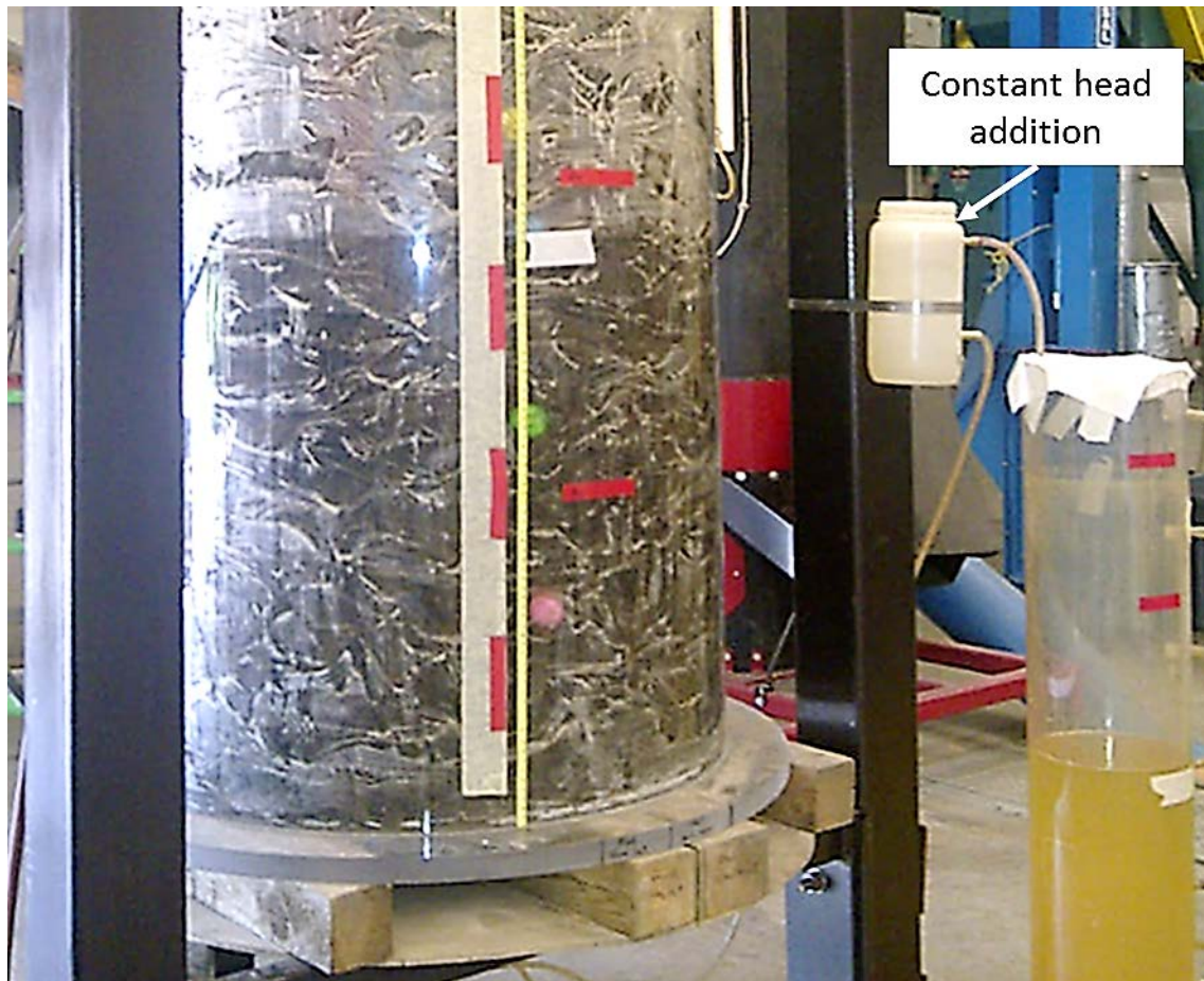
FIG. 7 Draining porosity test in progress showing the constant head addition (container) for collecting delayed drainage during draining porosity
