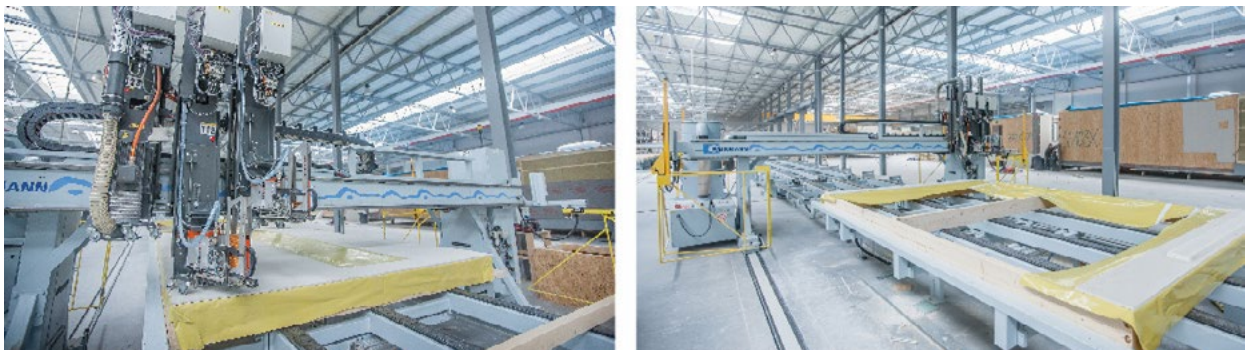
Figure 3. Nailing bridge. Photographs credits: Nordhus. Included with permission.
