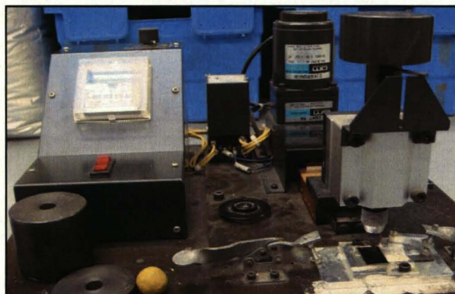
Figure 3-8 Specialised wear testing machine.
