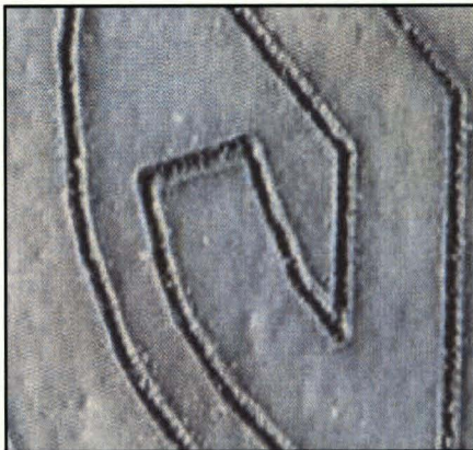
Figure 2-13 Photograph showing the laser mark produced by engraving mechanism[6].
