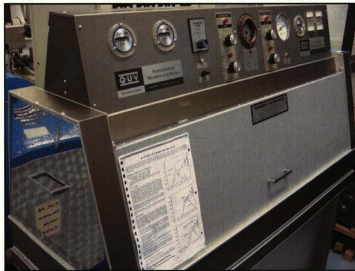
Figure 3-10 QUV Weathering Tester[28].
