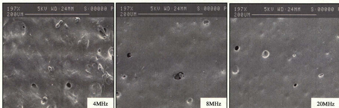
Figure 4-26 Micrographs showing the affect of frequency on contrast of BA1 grid marked samples at 250mm/s-1.
