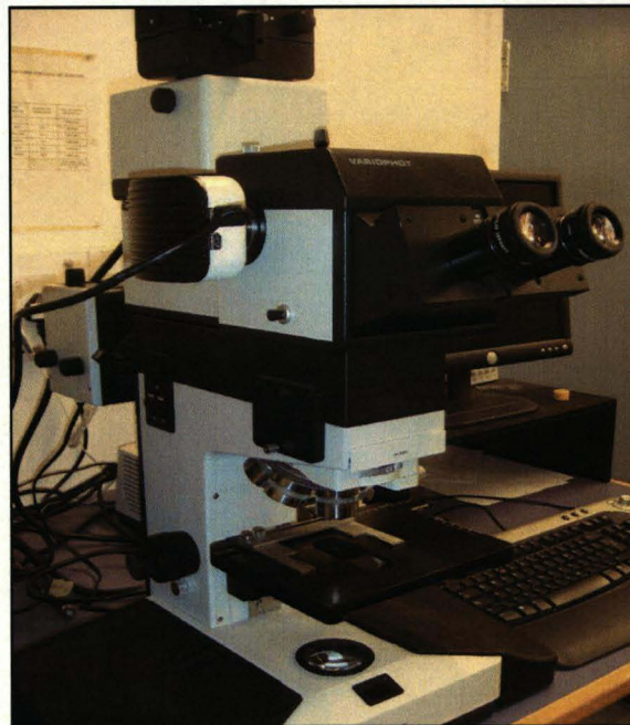
Figure 3-12 Leica Optical Microscope.
