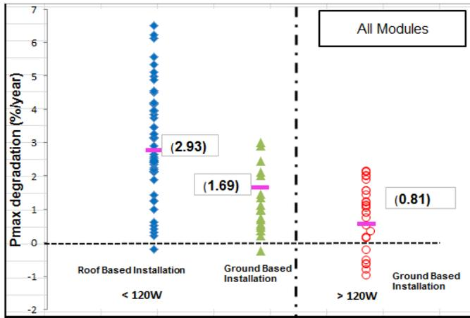
Figure 7. Effect of installation type on  $P_{max}$  degradation of all modules.
