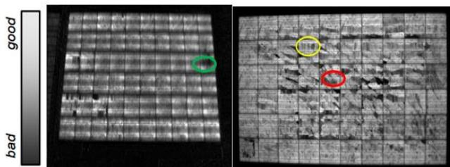
Figure 4. Electroluminescence images of some samples taken in the field.
