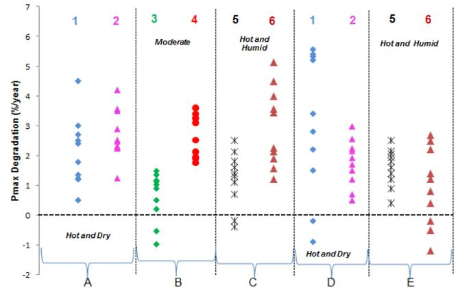
Figure 3. Site-wise, Manufacturer and climate-wise (Hot and dry, Hot and humid and Moderate)  $P_{max}$  degradation rates. 1 through 6 are different manufacturers with different colour representations
