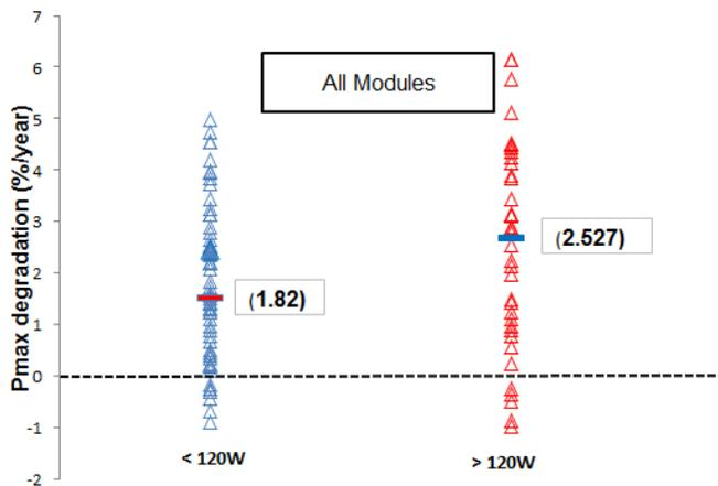
Figure 5. Effect of PV module size on  $P_{max}$  degradation of all modules.
