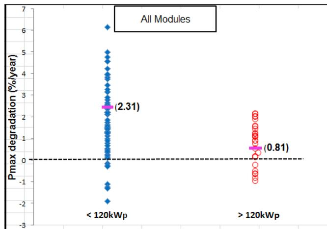
Figure 6. Effect of PV system size on  $P_{max}$  degradation of all modules.
