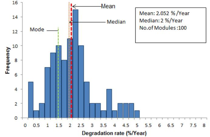
Figure 2. All modules  $P_{max}$  degradation histogram.
