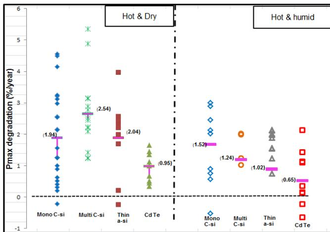
Figure 8. Effect of climate and type of PV technology on  $P_{max}$  degradation of all modules.
