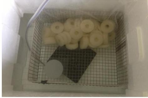
*Figure 1: Experimental set-up for the elution using megasonic sonication. The sponge filters, seen at the top of the figure have a doughnut shape when fully expanded and are enclosed in a plastic bag. The membrane is seen in a smaller bag on the bottom left of the figure. The megasonic transducer, seen as a black square, is placed at the bottom of the bath filled with water.*
