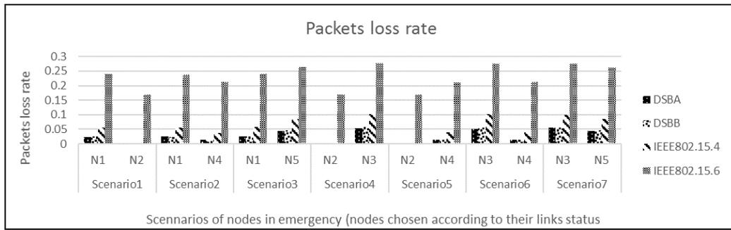
Figure 14: Packets loss rate for nodes in emergency applied in the seven scenarios at 1.875 ms slot length.
