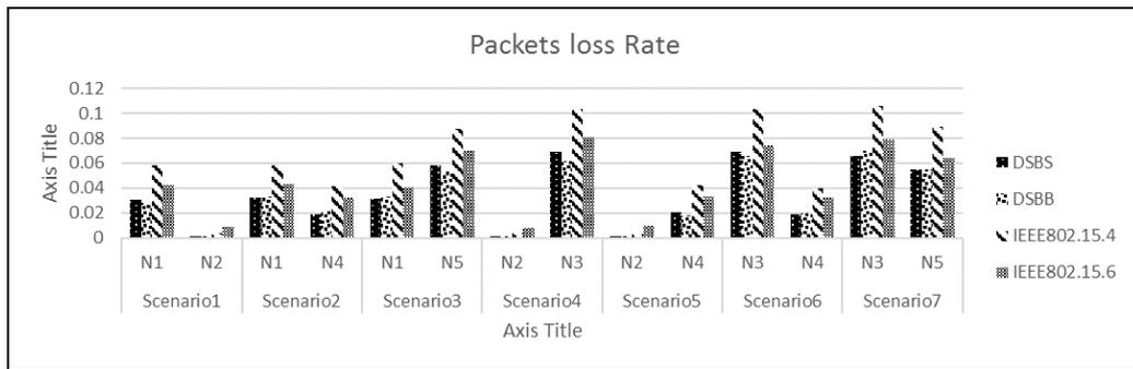
Figure 18: Packets loss rate for nodes in emergency applied in the seven applied scenarios at 7.5 ms slot length.
