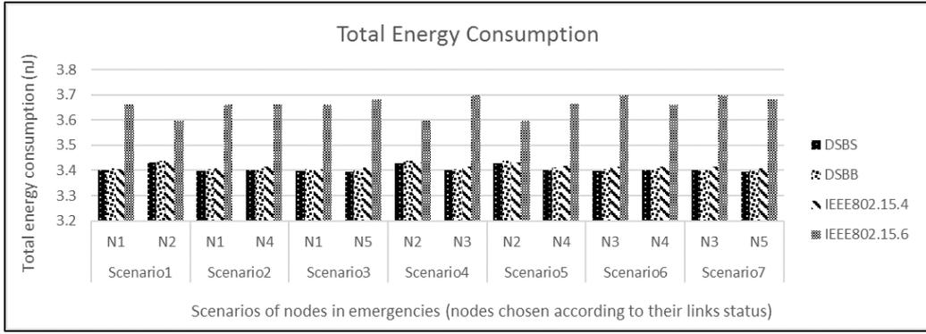
Figure 13: Total energy consumption with 3.75 ms slot length.
