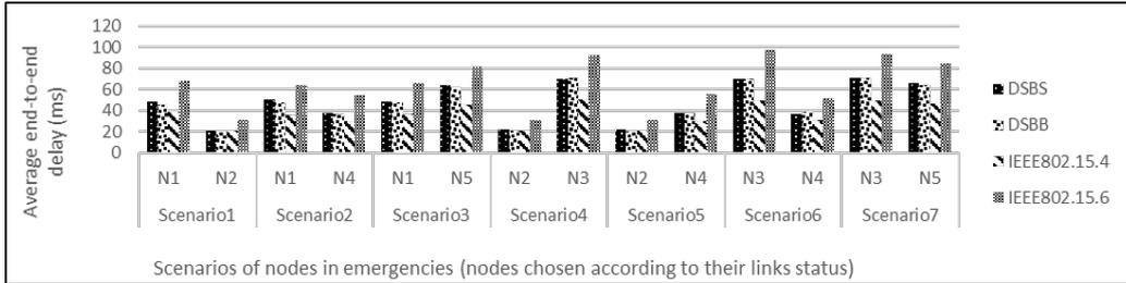
Figure 11: Latency for nodes in emergency with 3.75 ms slot length.
