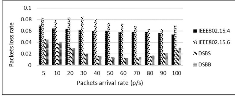
Figure 6: Packets loss rate for different and increasing CBR(s).
