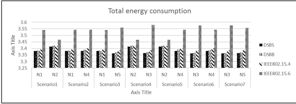
Figure 21: Total energy consumption for nodes in emergency at 7.5 ms slot length.
