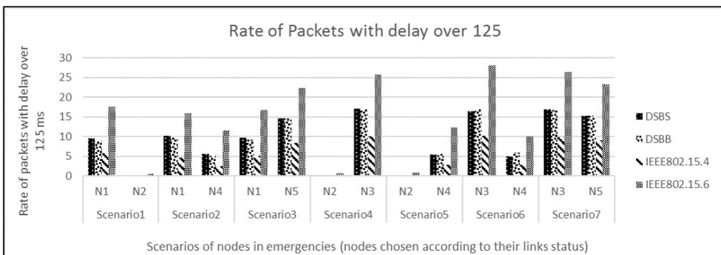
Figure 12: Rate of packets received with a delay over 125 ms with 3.75 ms slot length.
