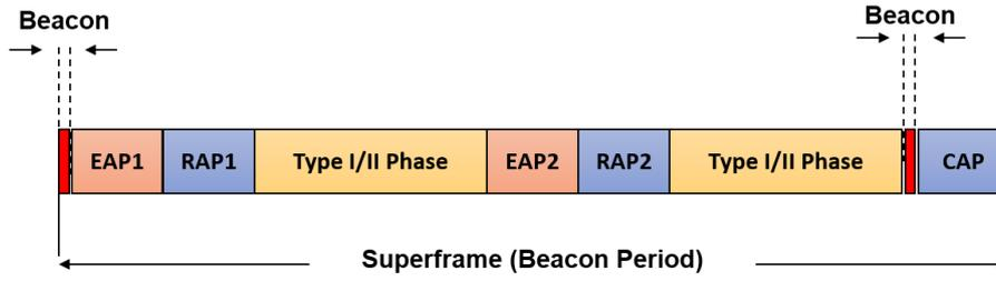
Figure 2: IEEE 802.15.6 beacon mode superframe structure.
