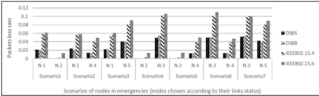
Figure 10: Packet loss rate with 3.75 ms slot length.
