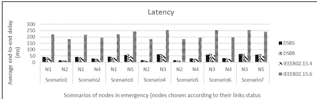
Figure 15: Latency for nodes in emergency applied in the seven applied scenarios at 1.875 ms slot length.
