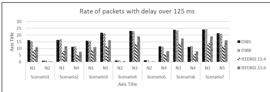
Figure 20: Rate of packets received with delay over 125 ms for nodes in emergency at 7.5 ms slot length.
