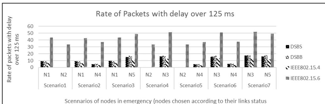
Figure 16: Rate of packets received with delay over 125 ms for nodes in emergency at 1.875 ms slot length.
