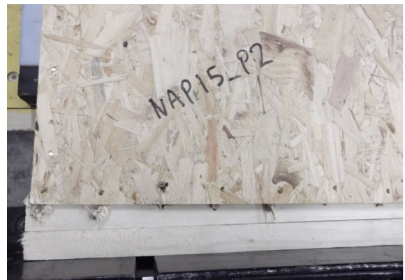
Failure observed in P7-P8
