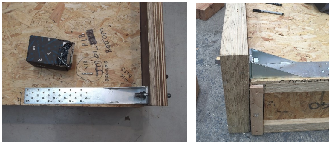
Figure 4-16 Holding down metal strap to plywood (left) and to KERTO (right) prior to fully restrained the panel to the rig.
