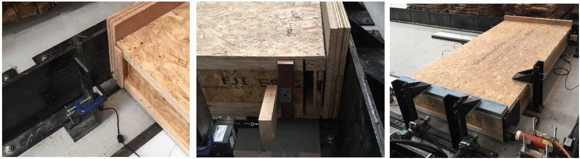
Figure 4-18 Transducers to measure displacement and horizontal racking load cell
