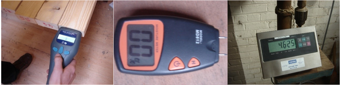
Figure 4-7 Equipment used for grading: MTG grader (left), moisture meter (middle) and scale (right)
