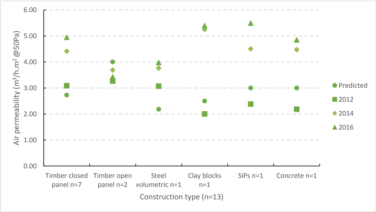
Figure 11: Construction type comparison of air permeability results
