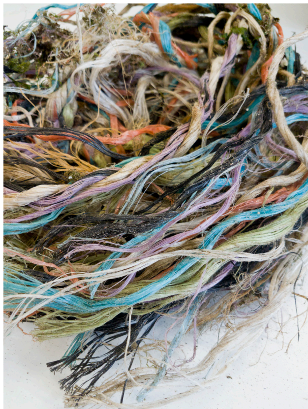
Fig. 2: Example of recovered rope plastic waste that was subsequently turned into Ocean Plastic PLA..
