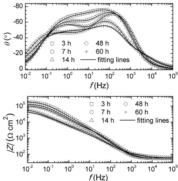
Fig.2 Impedance spectra of Ni-P\alginate microgels coatings recorded after 3-60 h of immersion in  $0.5 \text{ mol dm}^{-3}$  NaCl solution. Solid lines represent the calculated spectra.
