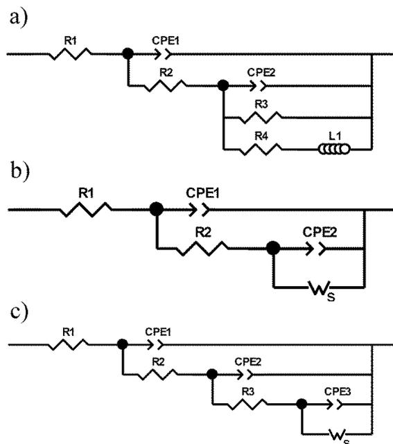
Fig.3 Models of equivalent circuits proposed for curve fitting of EIS data: a) model 1:  $R_1(CPE1[R_2(CPE2[R_3[R_4 L_1]])]])$ ; b) model 2:  $R_1(CPE1[R_2(CPE2 W_s)])$ ; c) model 3:  $R_1(CPE1[R_2(CPE2[R_3(CPE3 W_s)])])$ .
