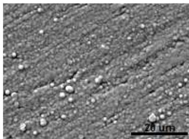
Fig.1 Scanning electron microphotograph of Ni-P coating with alginate based microgels.
